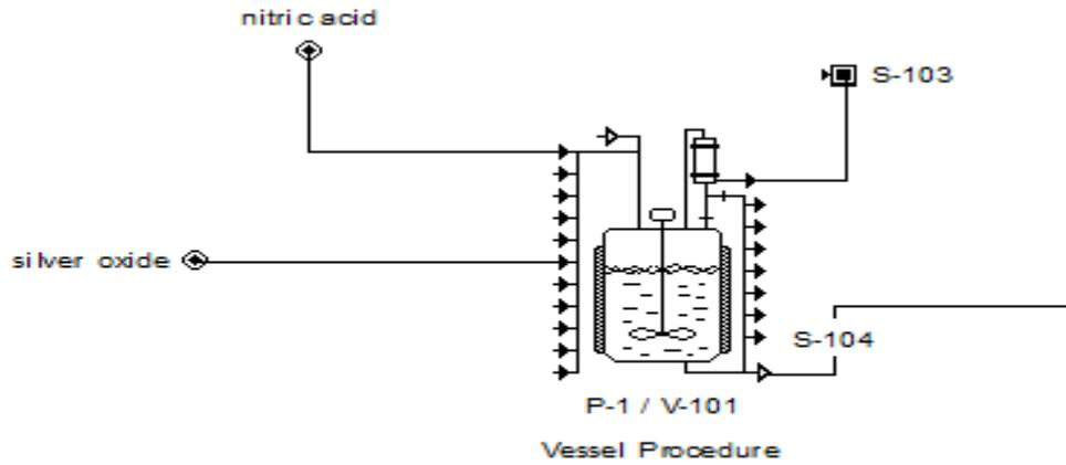
Figure 4.2 Batch reactor
