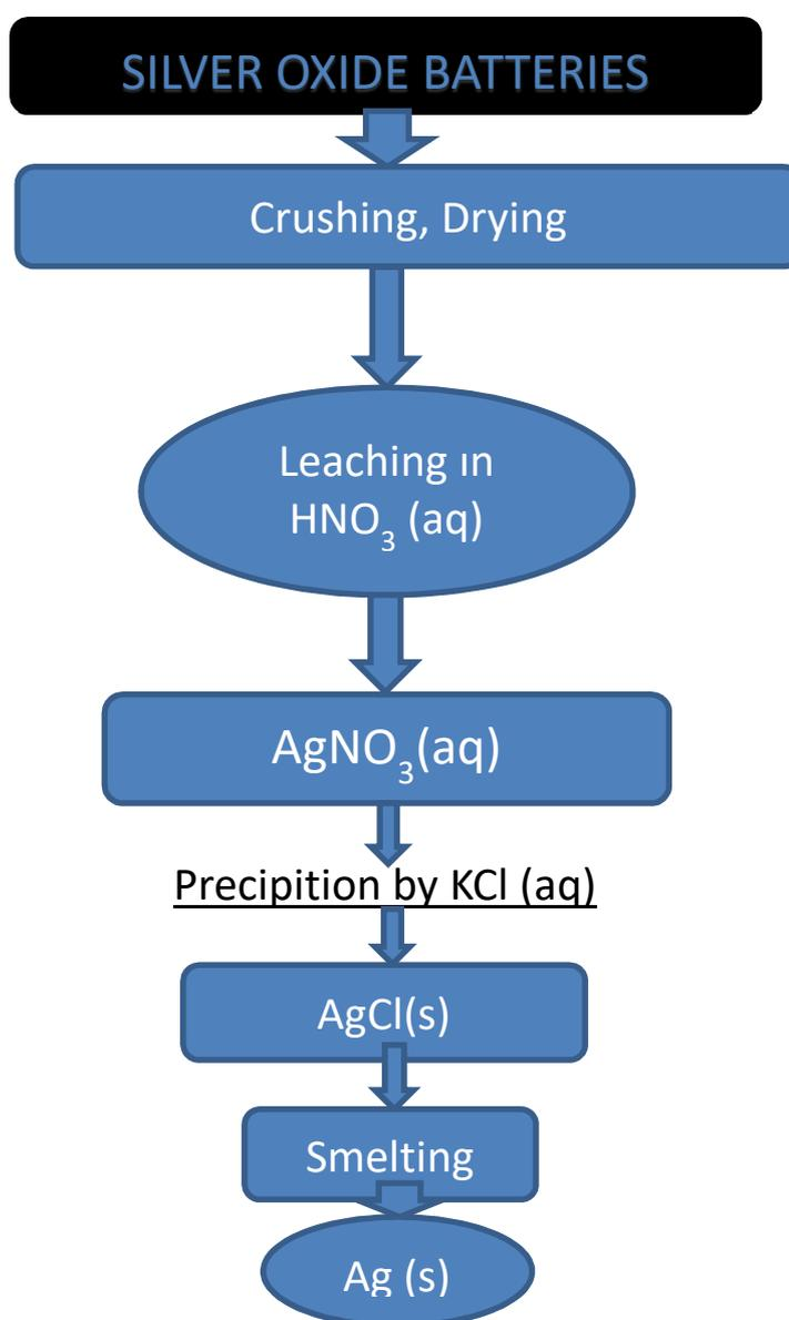
Figure 2.2 Precipitation by KCl
