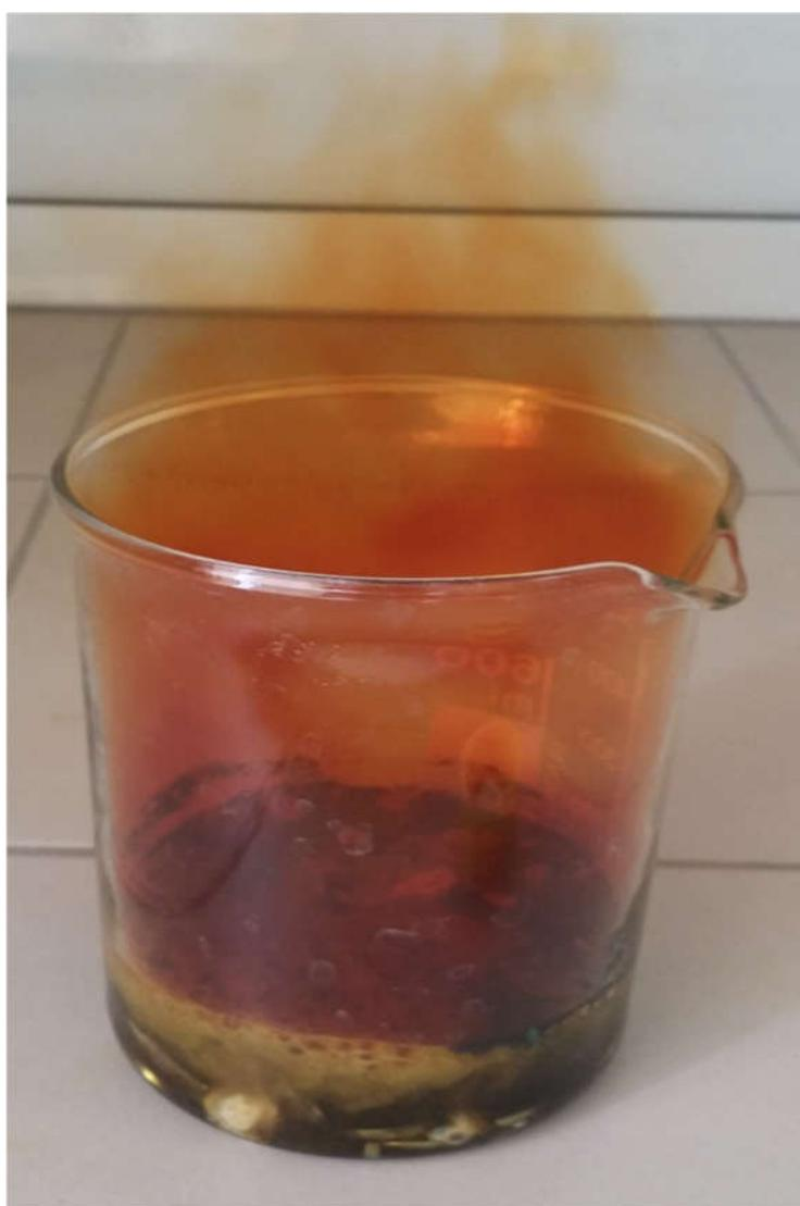
Figure 3.1 Addition of nitric acid to crushed silver oxide batteries.
