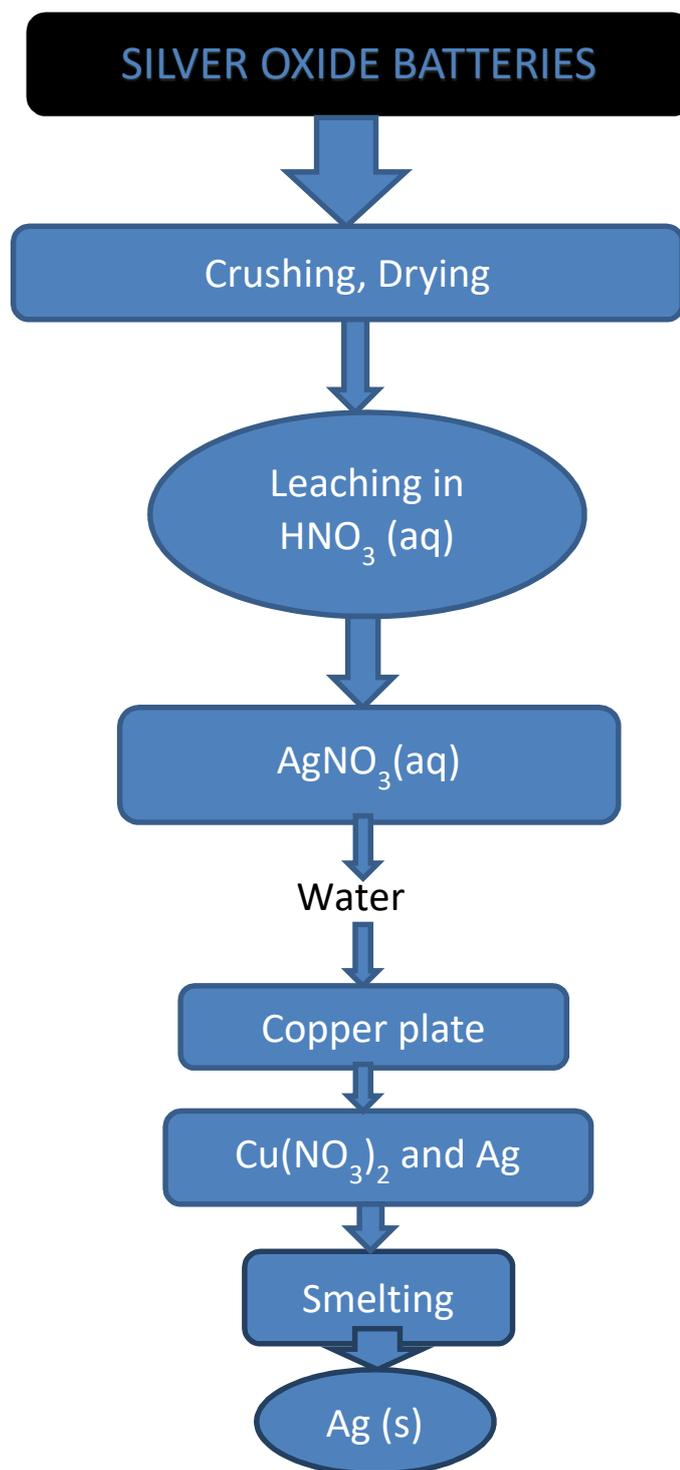
Figure 2.1 Precipitation by copper plate
