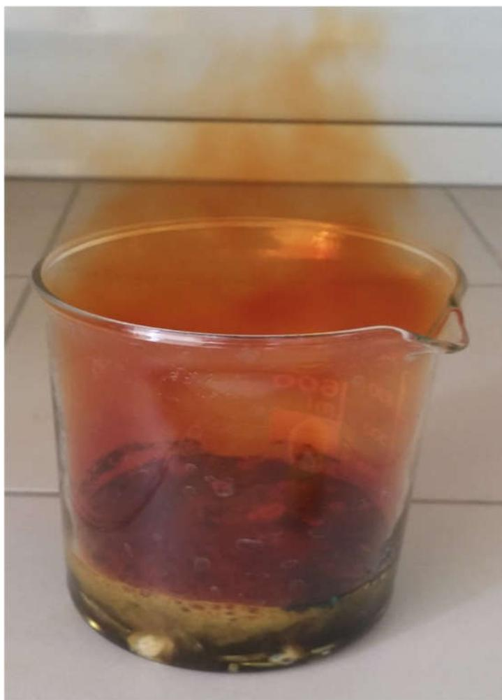
Figure 3.5 Dissolution of crushed silver oxide batteries in nitric acid.
