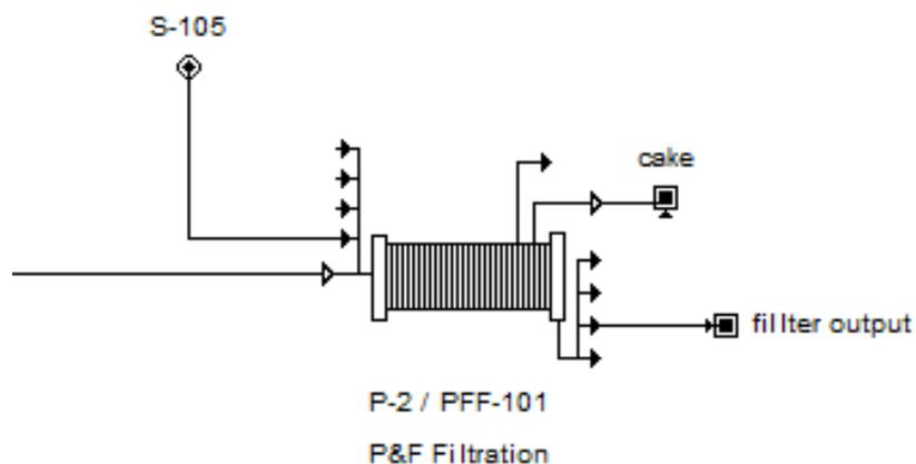
Figure 4.3 Microfiltration (feed and bleed operation).
