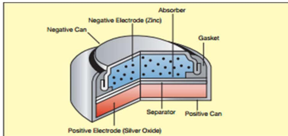
Figure 2.3 Battery construction [33].
